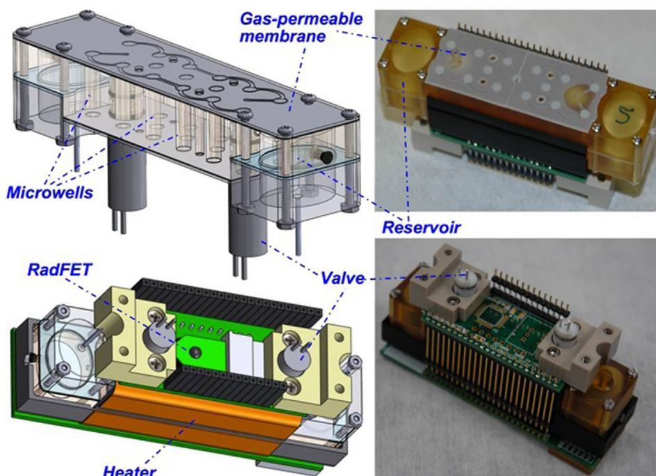
**Fig. 4.** Four different views (solid model at left, photographs at right) of one of three bioblocks included in the SESLO payload. The two valves protrude down from the block (upper left); reservoirs are the elliptical structures at both ends of the block; heater is orange and RadFET is a black dot near the center of the bottom left depiction. (For interpretation of the references to colour in this figure legend, the reader is referred to the web version of this article.)
