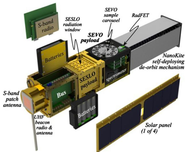
**Fig. 3.** The O/OREOS spacecraft showing key components, the bus and 2 payload cubes, and the NanoKite de-orbit mechanism that is helping O/OREOS's orbit decay from 650 km in  $\sim 22$  years [3,4].
