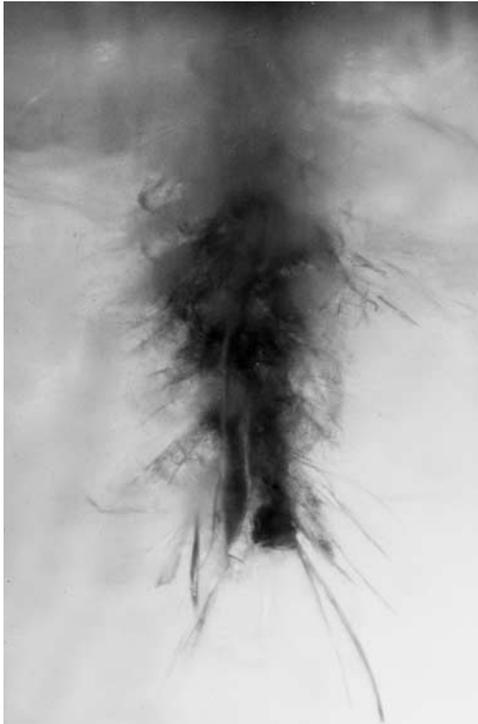
**Figure 3.** Intact capture in high-density aerogel with characteristic forward fracture lines.
