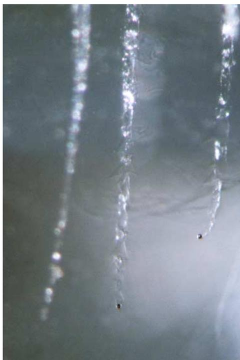
**Figure 5.** Intact capture in low-density aerogel shows typical long track with the particle arrested at the end of a curved hook.
